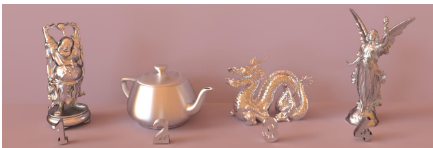
Fig. 14: Our method can handle different kinds of glossy materials: (1) Buddha: modified Phong BRDF with a shininess n=80 , (2) teapot: Ward anisotropic BRDF model with \alpha_x = 0.1 and \alpha_y = 0.5 , (3) dragon: pure specular, rendered with a path tracing technique (4) Lucy: a Micro-facet based BRDF model (with a Beckmann distribution \alpha = 0.2 ), the ground and the back wall are Lambertian.
