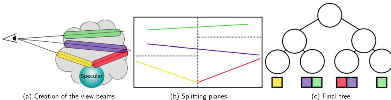
**Fig. 3** Example of a view beam Kd tree building for a set of beams (a). Only the supporting rays are used in the tree (b). Some leaves (c) contains several beams, and beams crossing splitting planes are duplicated in the tree
