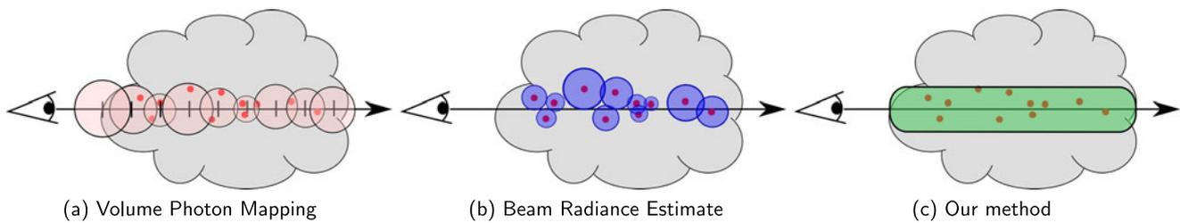
**Fig. 1** Different ways to gather photons. Regular ray marching (a) may take into account several times a same photon whereas *Beam Radiance Estimate* (b) and our method (c) gathers all photons once and for all
