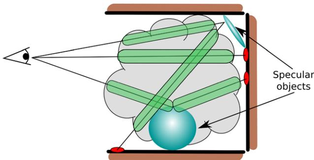
**Fig. 2** Different possible view rays in a scene. The rays going through the medium have view beams (in green) associated, and visible points (in red) are created on diffuse surfaces
